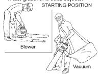
AWARNING: When starting engine, hold the unit as illustrated. Do not set unit on any surface except a clean, hard area when starting engine or while engine is running. Debris such as gravel, sand, dust, grass, etc. could be picked up by the air intake and thrown out through the discharge opening, damaging the unit or property, or causing serious injury to bystanders or the operator.
